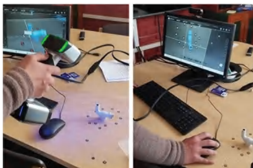
Figure 2: Three dimensional (3D) scanning process of faucet.
