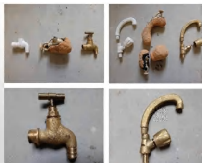
Figure 3: Brass faucets after casting.
