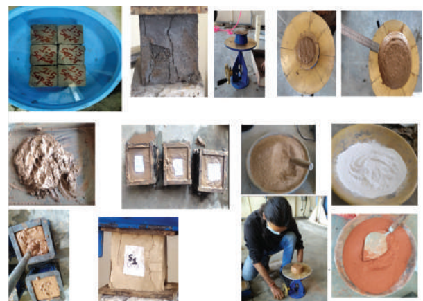
Figure 2: Preparation of mortar cubes mud and others.
