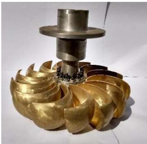
Manufactured Brass Runner
