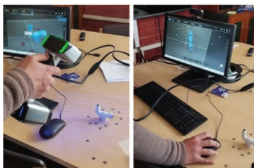
Figure 2: Three dimensional (3D) scanning process of faucet.
